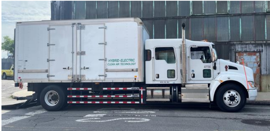
An older city-owned box truck that has been retrofit with sideguards.
